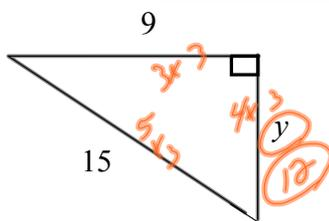
$$\begin{aligned} y^2 + 9^2 &= 15^2 \\ y^2 &= 15^2 - 9^2 \\ \sqrt{y^2} &= \sqrt{144} \\ y &= 12 \end{aligned}$$
