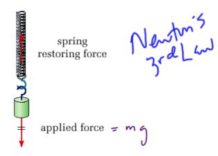
Hooke's Law: The applied force or restored force is directly proportional to the extension or compression of a spring.
