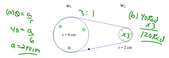
Ex. A small electrical motor turns at 2200 rpm.
