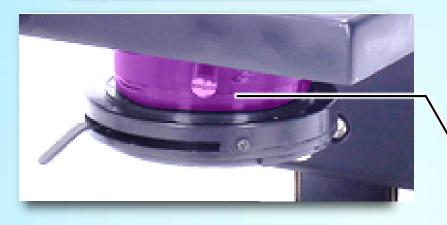
The lens under the stage that <u>focuses light</u> from the illuminator through to the <u>hole</u> in the stage.
