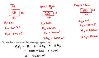
Step 2) Storage space consist of 3 walls and a roof (3m x 6m x 5m)
