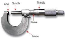
The value on the sleeve represents millimetres and the value on the thimble represents hundredths of a millimetre.
